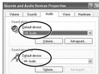
If another device is selected, use the "Default Device" pull-down menu to change the selection to "H4 Audio". When the setting has been made, click the OK button to close the sounds and audio devices properties screen.
